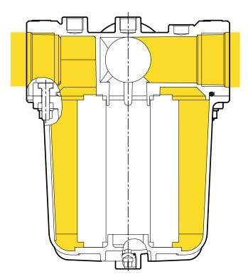
Figure 6 Mod 50000 cartridge filter
